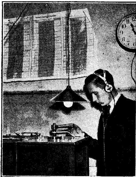
The "Brussels" wavemeter in use at Tatsfield. An important part was played by the B.B.C. checking station during the wavelength change-over.
