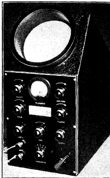
Ediswan cathode-ray oscillograph.
